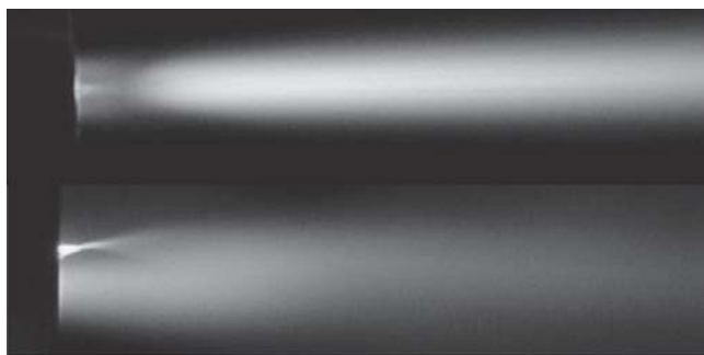
Fig. 1 Centered and off-centered wire positions within the spray hardware
